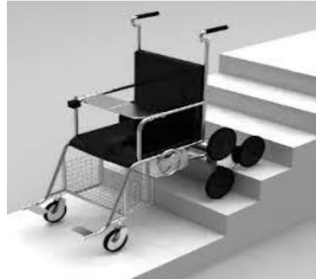
Figure 5. Wheel Chair that can be used on the Staircase
