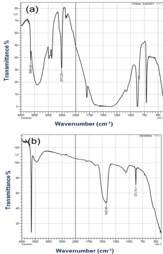
**Figure 3.** FTIR spectra of (a) ground duck eggshells powder (DES) and (b) calcined duck eggshells powder at 900 °C (DES-900)
