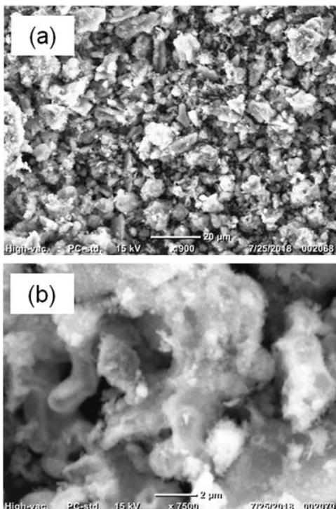
**Figure 5. (a) Lower and (b) higher magnification SEM images of Mg-incorporated HAp sample prepared at room temperature (Mg-HAp)**
