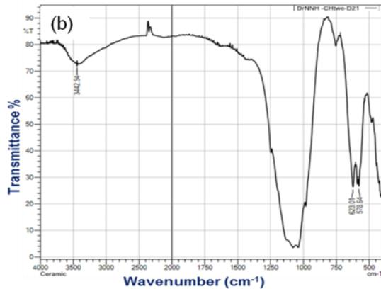
**Figure 4(b).** FTIR spectrum of Mg-incorporated HAp samples prepared at 40 °C (Mg-HAp-40)
