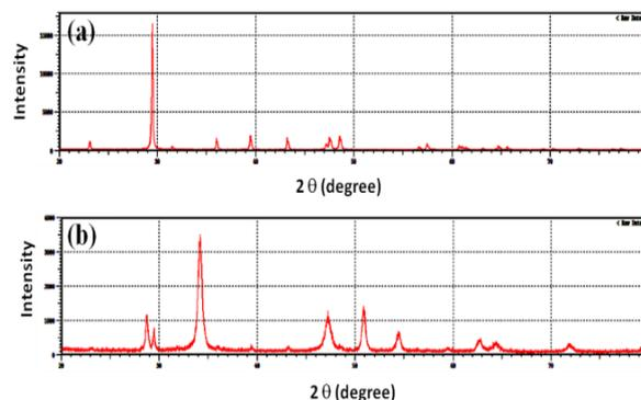
**Figure 1. XRD patterns of (a) ground duck eggshells powder (DES) and (b) calcined duck eggshells powder at 900 °C (DES-900)**
