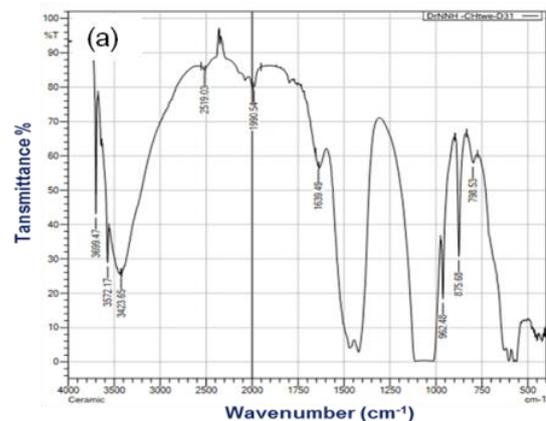
**Figure 4(a).** FTIR spectrum of Mg-incorporated HAp samples prepared at room temperature (Mg-HAp)
