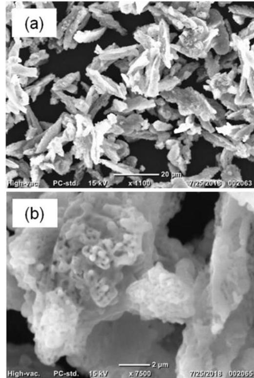
**Figure 6. (a) Lower and (b) higher magnification SEM images of Mg-incorporated HAp sample prepared at 40 °C (Mg-HAp-40)**
