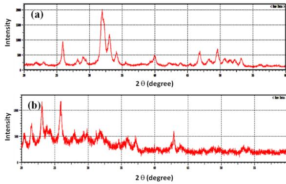
**Figure 2.** XRD patterns of Mg-incorporated HAp samples prepared (a) at room temperature (Mg-HAp) and (b) at 40 °C (Mg-HAp-40)
