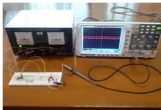
Figure 5. Testing astable frequency generator circuit
