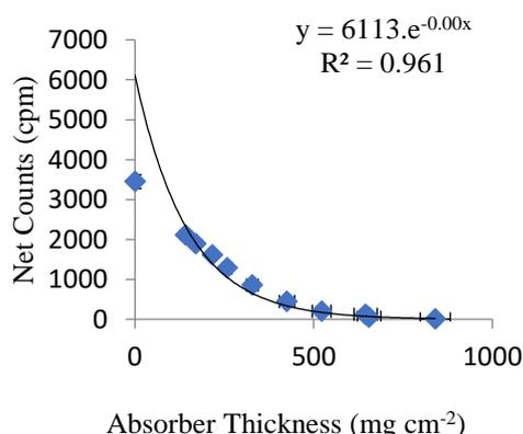
**Figure 3. The Standard Absorber Calibration Curve (Exponential Fitting)**
