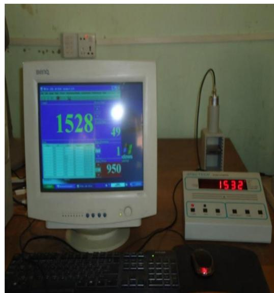
**Figure 2. The Measurement Condition for Experimental Setup of Geiger-Muller Counter (ST-360)**
