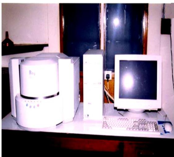
**Figure 6. Photograph of spectrometer (Shimadzu EDX-720)**
