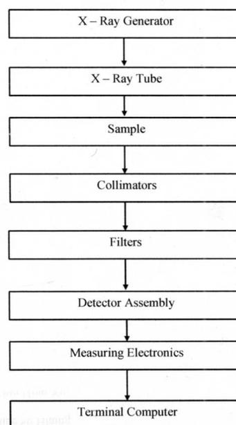
**Figure 5. Schematic diagram of X-ray spectrometer**
