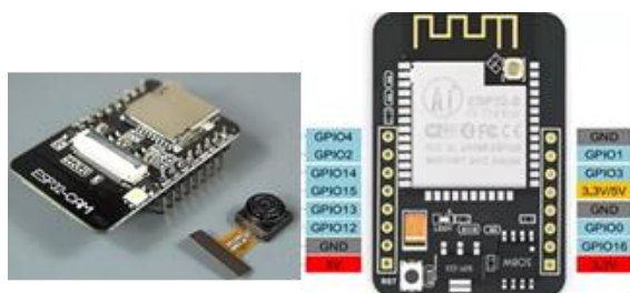
Figure 2. ESP32_CAM and its pin diagram
