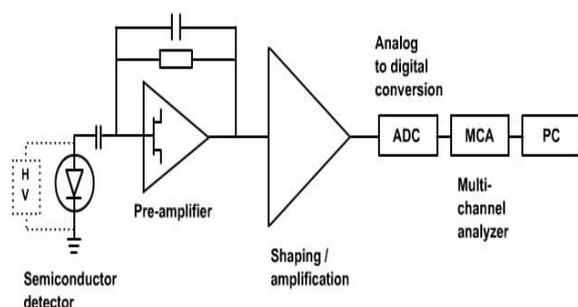
**Figure 1. Block diagram of electronic set-up of EDXRF system**
