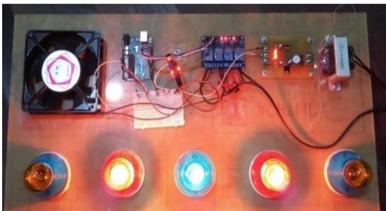
**Figure 12. Light bulbs 2, 3, 4 ON and bulb 1 OFF after 2 claps**
