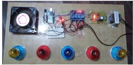
**Figure 14. Fan ON and bulb 4 OFF after 4 claps**
