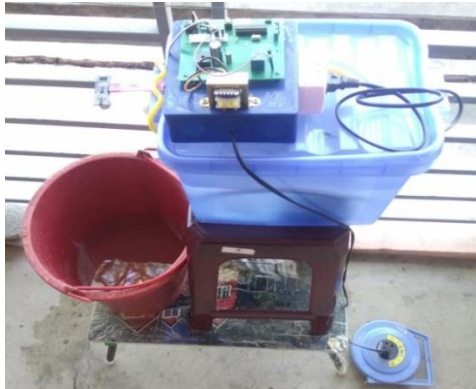
Figure 10. Photograph of the developed automatic water dispenser
