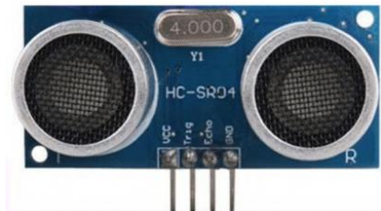
Figure 2. Photograph of HC-SR04 ultrasonic sensor
