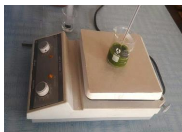
Figure 4. Photograph of papaya solution are heated and stirred with magnetic stirrer
